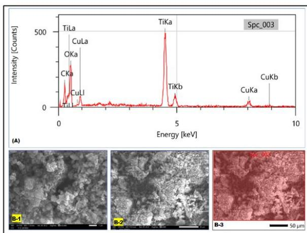
Figure 3: Characterization of Cu-doped TiO<sub>2</sub> nanocomposites (A) EDX Spectra; (B 1-3) SEM image taken at 500X magnification.
