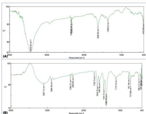
Figure 5: FTIR characterization of Cu-doped TiO<sub>2</sub> nanocomposites
