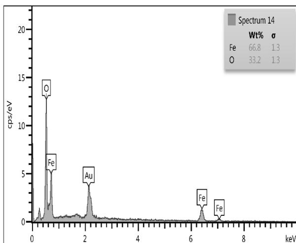
Figure 4: E.D.X. of Fe<sub>3</sub>O<sub>4</sub>
