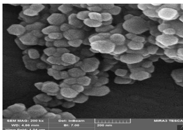
Figure 5: S.E.M. of Fe<sub>3</sub>O<sub>4</sub>
