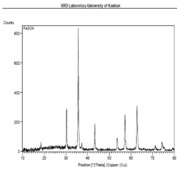
Figure 2: XRD of Fe<sub>3</sub>O<sub>4</sub>
