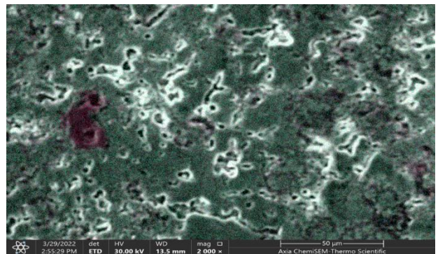
Figure 4: Scanning electron microscopy (FeSem) image of base ingot (A5) at constant pressing pressure (600Mpa).
